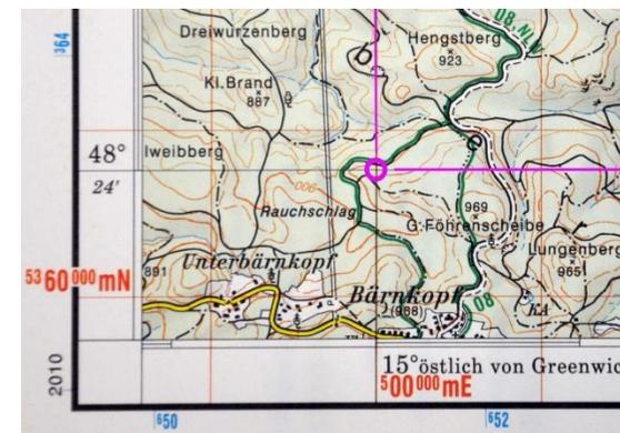
Figure 29-4 Relation between the sheet lines and the map border, resulting in an overlap with the adjoining sheets.
